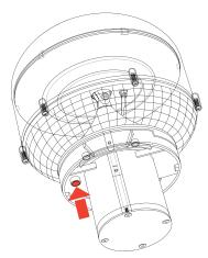
When installing the ground mount base, please put Part A and Part B into the ground holes first then install the ground mount base on top.
