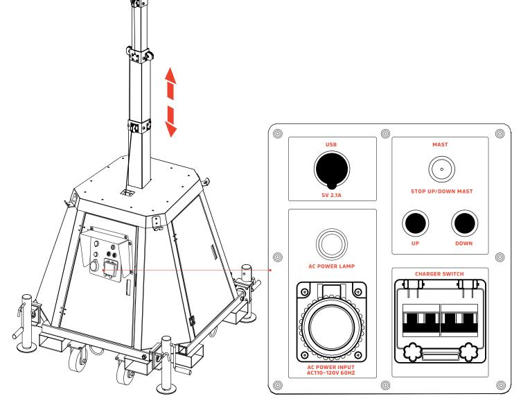
Press the UP and DOWN buttons on the control board to adjust the pole height.
