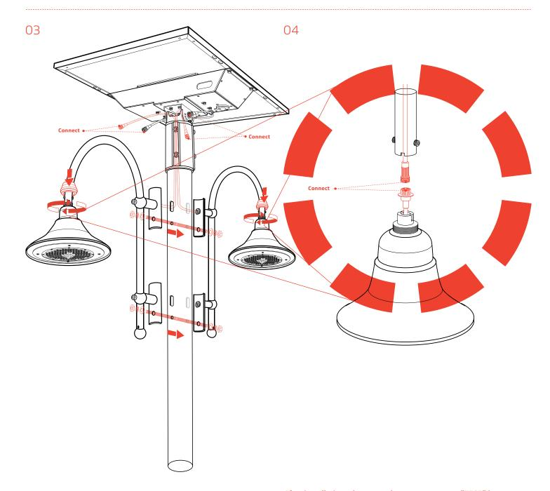
After installation, please use the program remote "TEST" button feature to ensure successful light fixture functionality. You may then select the preferred operating mode to complete the setup.
