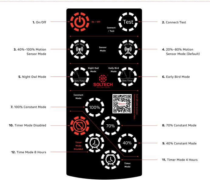
The range of the remote control to the indicator is 16ft (Day time) to 33ft (Night time). Because the sunlight will impact the signal of the remote control, we suggest our users to setup the mode before they install the light.
