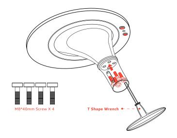
Place the light head on top of the pole and tighten the two M8\*16mm screws by T shape wrench into proper position.
