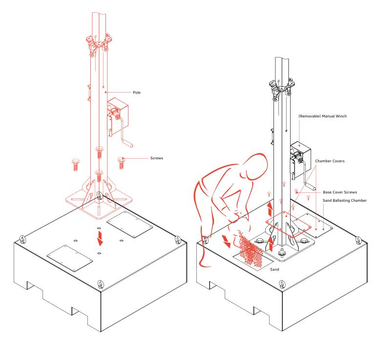
Install the pole on the base with pole screws.
