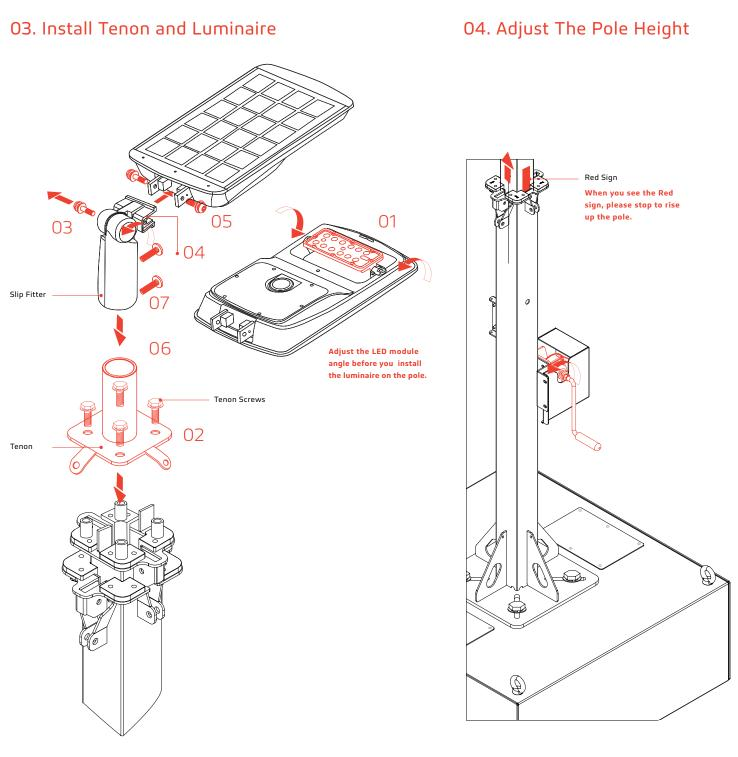
Install Tenon and Luminaire on the top of the pole.
