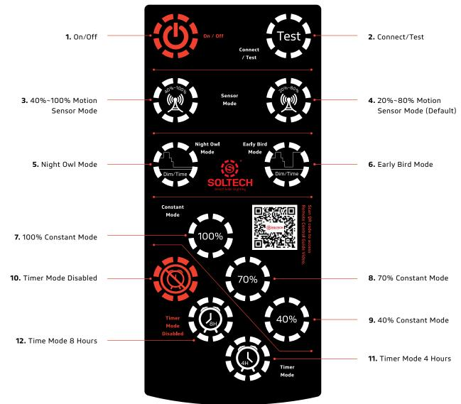
The range of the remote control to the indicator is 16ft (Day time) to 33ft (Night time). Because the sunlight will impact the signal of the remote control, we suggest our users to setup the mode before they install the light.
